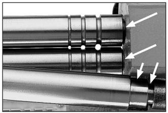
Figure 44. T21323 lubrication locations (right side shown).
